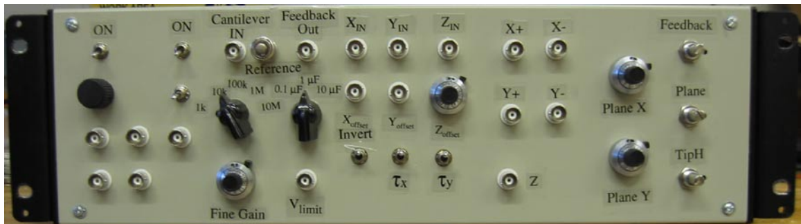
Figure 2.22 Picture of the new box containing the plane fitting electronics and the cantilever feedback circuit. The inputs and outputs are labeled with their function.
