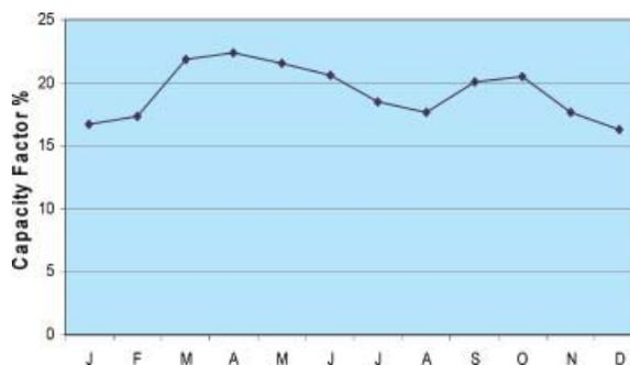
Figure 10. Average monthly capacity factor for Springerville systems
