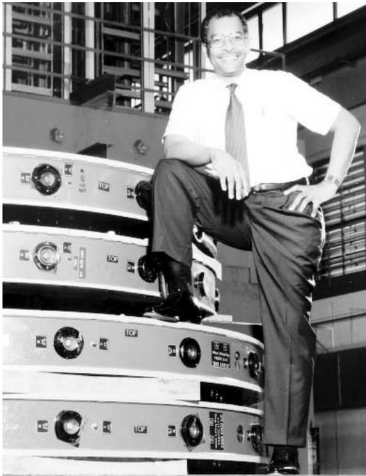
Fermilab physicist Herman White, with photon veto counters for KTeV, before their installation in the experiment's beamline. The veto counters reject particles at very large angles to the beam line, to rule out false decay signals.
