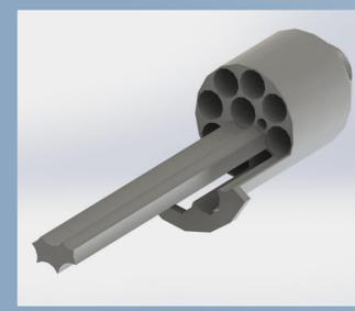
**Figure 5:** SolidWorks rendering of cartridge able to hold 9 mL liquid samples centered within the MRI coil.
