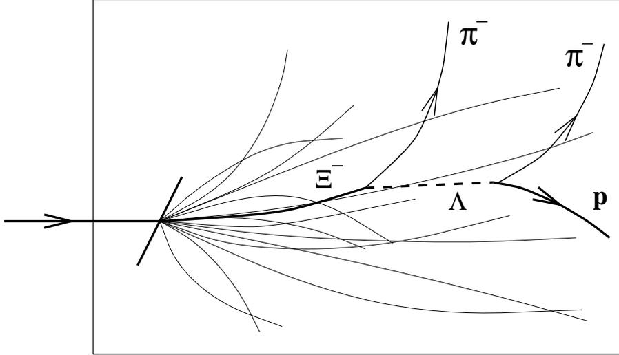
Figure 2: Schematic representation of the  $\Xi^-$ -decay topological structure showing as dashed line the invisible  $\Lambda$  emerging from the decay kink and the decay ‘V’ of the final state charged particles. Other directly produced charged particle tracks propagating in a magnetic field normal to the figure plane are also shown.
