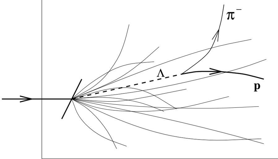
Figure 1: Schematic representation of the  $\Lambda$ -decay topological structure showing as dashed line the invisible  $\Lambda$  and the decay ‘V’ of the final state charged particles. Other directly produced charged particle tracks propagating in a magnetic field normal to the figure plane are also shown.
