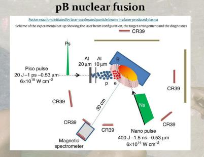
The long-pulsed nano-laser produces plasma and sweeps electrons away. The short-pulsed pico-laser produces a beam of reactant protons. Fusion reactions occur prior to protons reaching thermal equilibrium.
