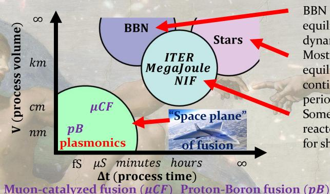
BBN in a homogenous thermally equilibrated plasma which is dynamic and expands over time. Most stellar nucleosynthesis is an equilibrium process which is continuous and stable over large periods of time. Some larger manmade fusion reactors are designed to operate for short pulsed periods of time.
