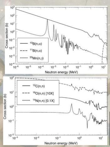
The collision cross-section of 14 MeV neutrons in matter is typically 10 times (or more!) smaller compared to MeV neutrons. Therefore, the neutron energy declines slowly from collisions (moderation). Containment walls must then be very thick. Much of the material is subject to element transmutation from exposure to such high energy and high intensity dt fusion neutrons.
