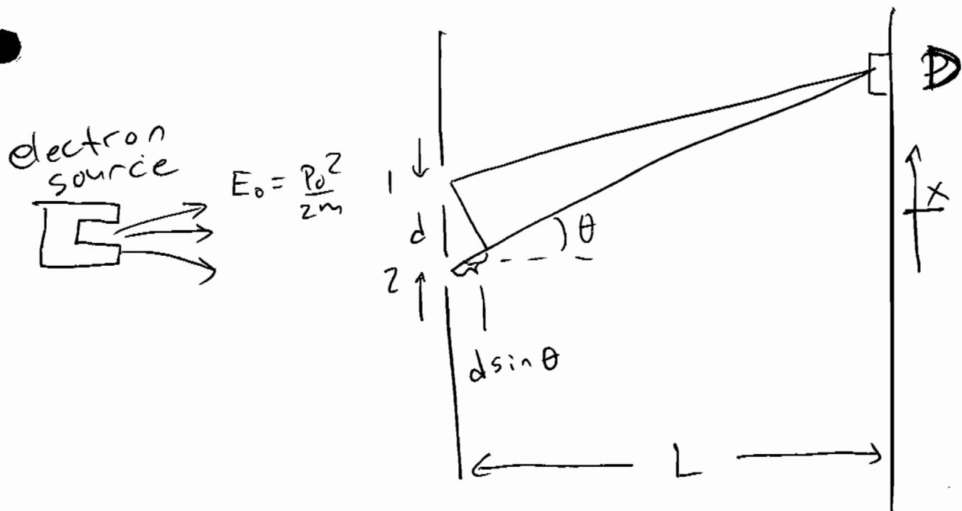
An electron gun emits electrons of energy  $E_0$  toward a screen with
