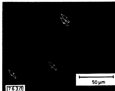
Fig. 1 Nomarski contrast photograph of an InP surface etched with HBr:H_3PO_4 solution (1:2) for 8s, revealing a significantly low EPD of \sim 10^6 \text{cm}^{-2}
