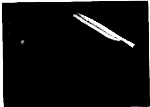
Fig. 1. An atomic force microscope image, obtained in the contact mode , of one single-shell (left-hand side) and two adjacent multi-shell nanotubes (right-hand side) on the oxidized Si(111) substrate.
